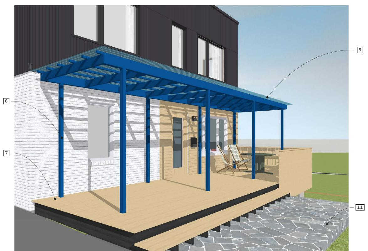
Metal porch structure painted color similar to Pantone 280C 8 3" square tube steel posts, 3x6 tube steel beams, 1 1/2" sq. purlins (pending structural review)
